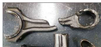
< Connecting rod broken >
